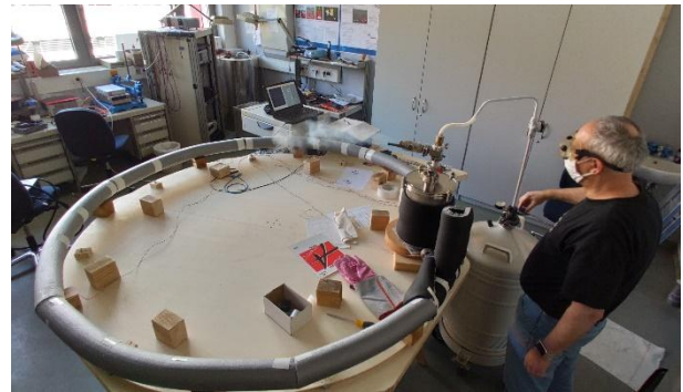
Figure 3: First laboratory prototype of a superconducting PP-coil.
