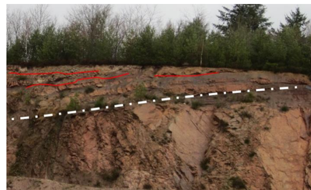
Figure 1. Picture of a man-made outcrop with – in red – bedding of the sedimentary deposit (sandstone) and – dotted white line – the geological limit between sandstone and the crystalline basement rock.
